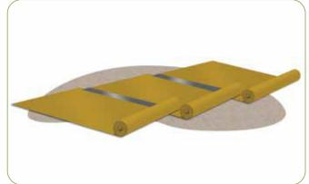
Figure 1. Radon Block™ Overlapping Roll-out Method
